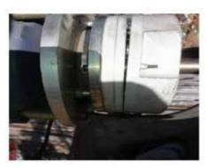
Typical case of stator resting bolt head, which will restrict the stator lateral movement of brake disc: This should be noticed and avoided during preventive maintenance.
